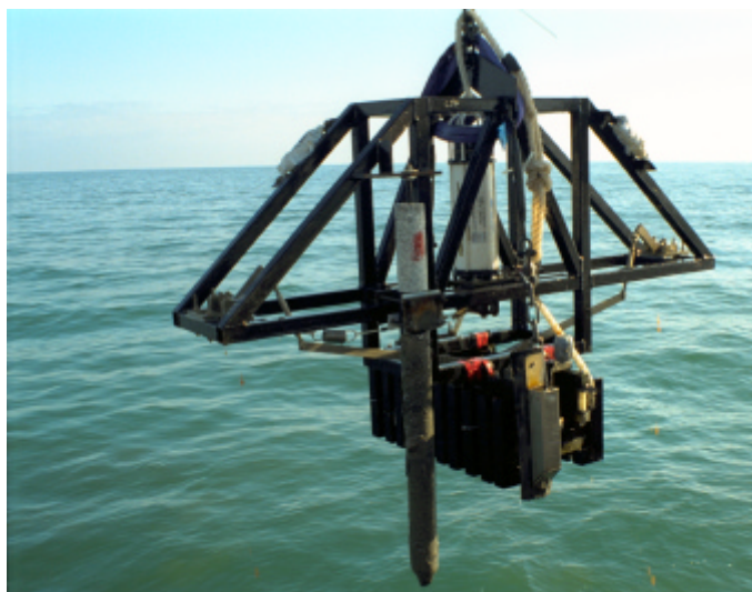
In-situ corrosion tests on pipeline materials
