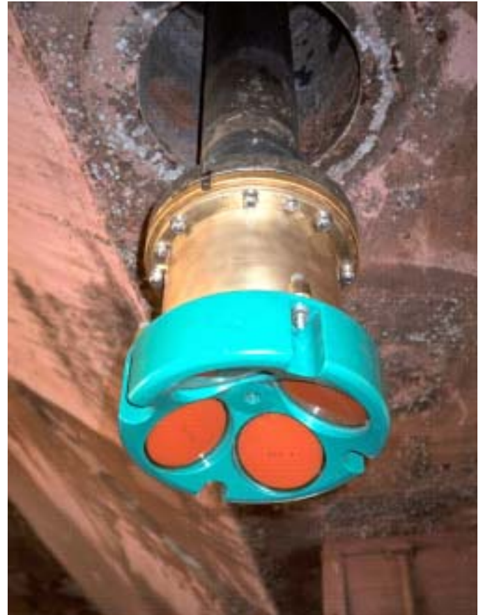
A Fugro SeisADCP installation
