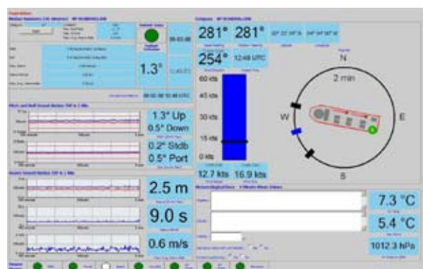
Helideck motion monitoring vessel display
